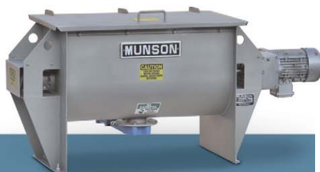
RIBBON/PADDLE/PLOW BLENDERS HANDLE POWDERS TO PASTES
