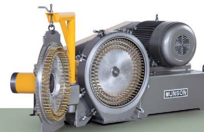
PIN MILLS REDUCE FRIABLE SOLIDS IN CONTROLLED SIZE RANGES
